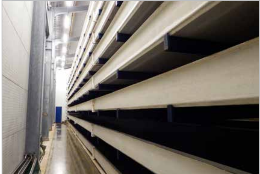
Multi-layer turbot farming at Seafarm B.V. The fishes are grown in these vertically stacked tanks, and moved from here through the processing and packing chain entirely using robotics. The farm also uses machinery to clean and maintain these vertical tanks.
